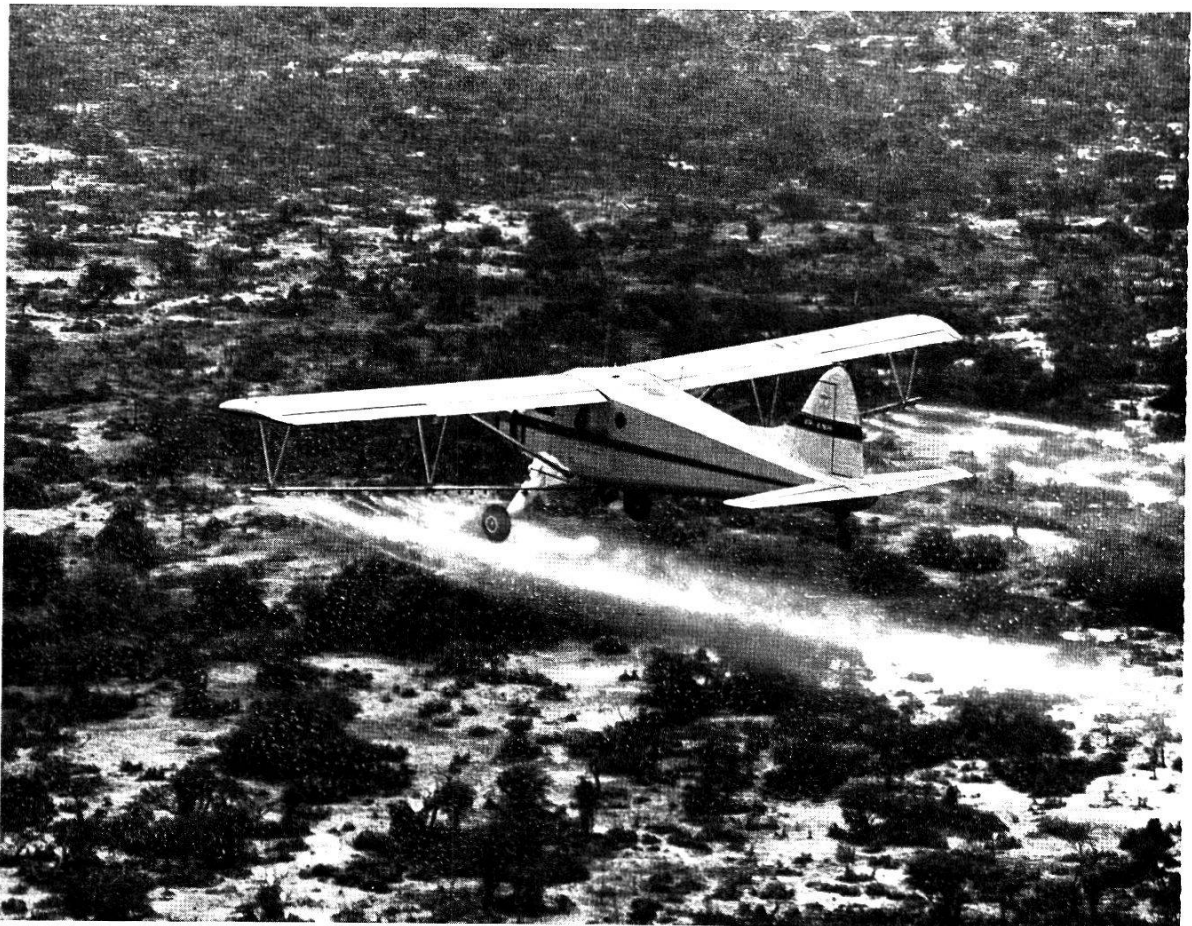
Fig. 61. A desert locust survey aircraft, fitted with boom and nozzle spray gear spraying a swarm in Somaliland.
