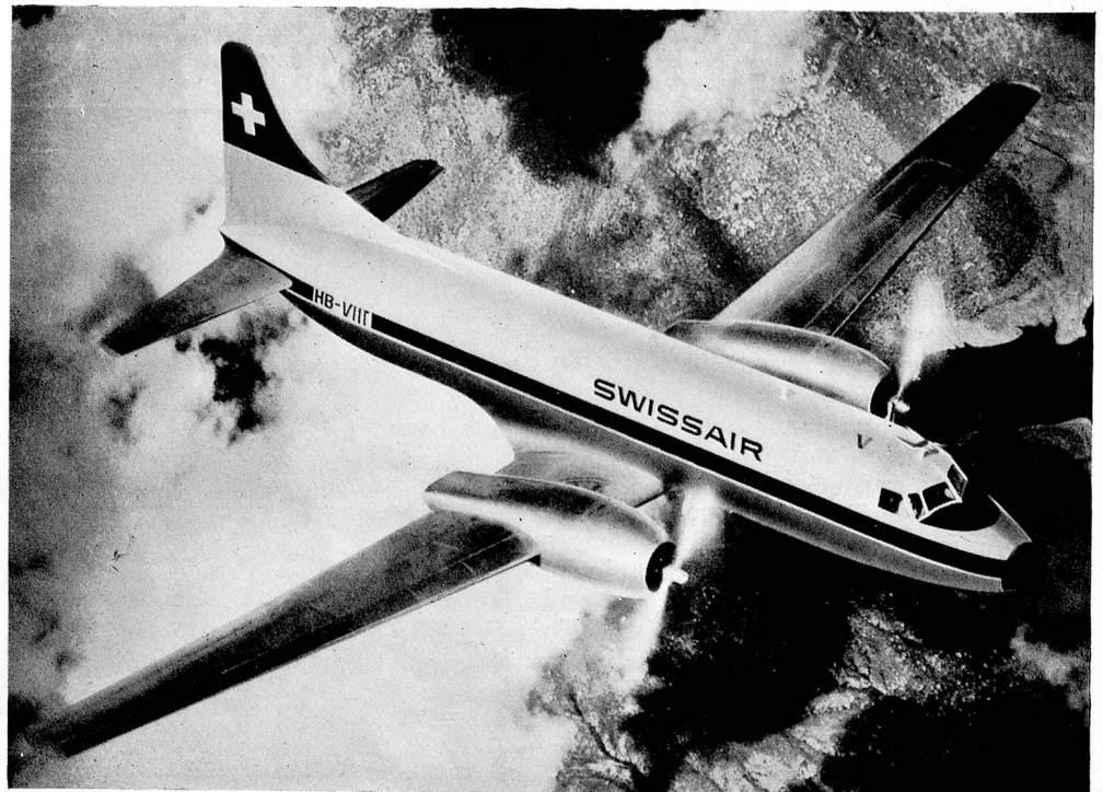
Soon to join Swissair's fleet: the new Convair "Metropolitan". Note the black-painted nose housing the weather-mapping radar.
