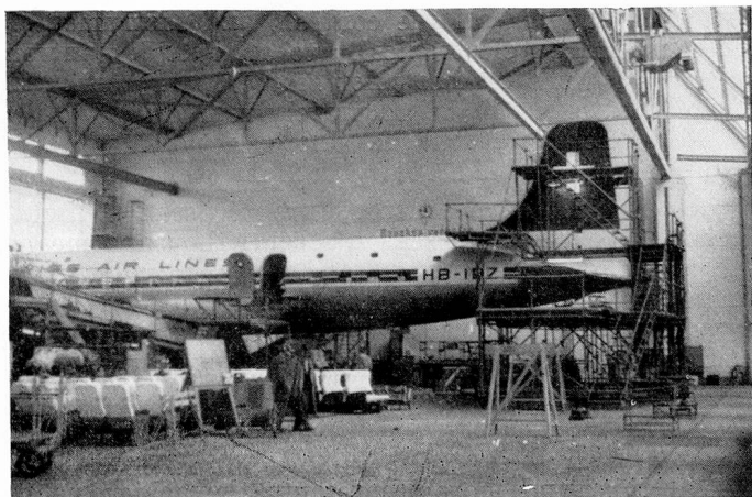
A Swissair plane in the maintenance dock where wings, fuselages and control surfaces are regularly examined and maintained.
