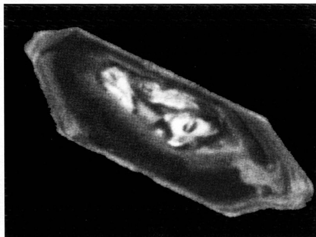
Fig. 4 CL image of a core-bearing zircon crystal belonging to population 63B; field of view: 180 \times 120 \mu\text{m} .
