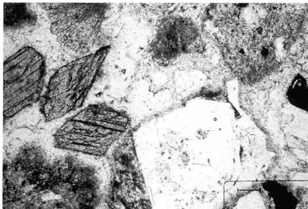
Fig. 3 Green and brown amphiboles in shallow water sandy marls (Pleistocene age) from Mt. Arkhangelos base; figure size: 2.6 mm across.
