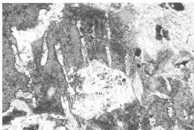
Fig. 3 Photomicrograph of hennomartinite overgrowing idiomorphic sugilite and serandite-pectolite needles. Width of the micrograph: 0.5 mm.
