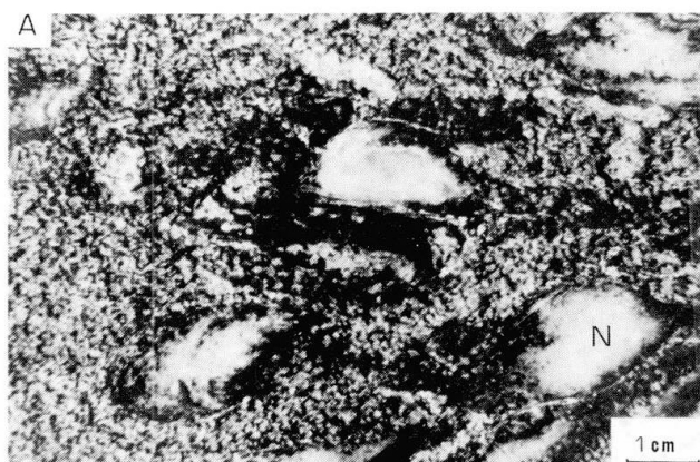
Fig. 4 Sample photograph showing the occurrence of fibrolite nodules in melanocratic gneisses perpendicular to the elongation of the nodules and perpendicular to the S_2 schistosity, horizontal in the photo. N = fibrolite nodules. (See text for explanation.)
