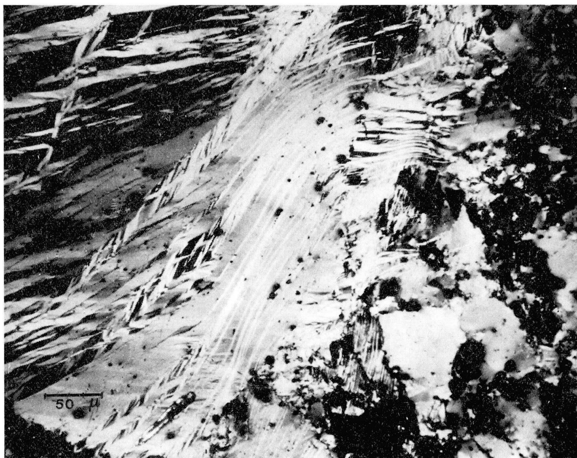
Fig. 5. Stibnite from Su Suergiu mine, deformed according to the open folds of the late tectonic phases. It shows undulatory extinction and twin-gliding parallel to the axial plane of the fold. Polished section, +N.
