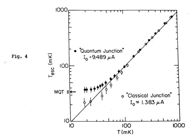
of the escape rate (solid dots). The escape rate becomes temperature independent at low temperatures which is expected if the escape mechanism is dominated by quantum fluctuations. This interpretation is supported by the quantitative agreement between this limit value of the measured escape rate and its theoretical prediction (arrow).
