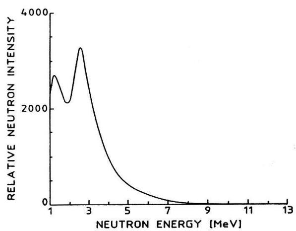
Fig.2: unfolded spectrum  $^{252}\text{Cf}$  source with NE-230 spectrometer
