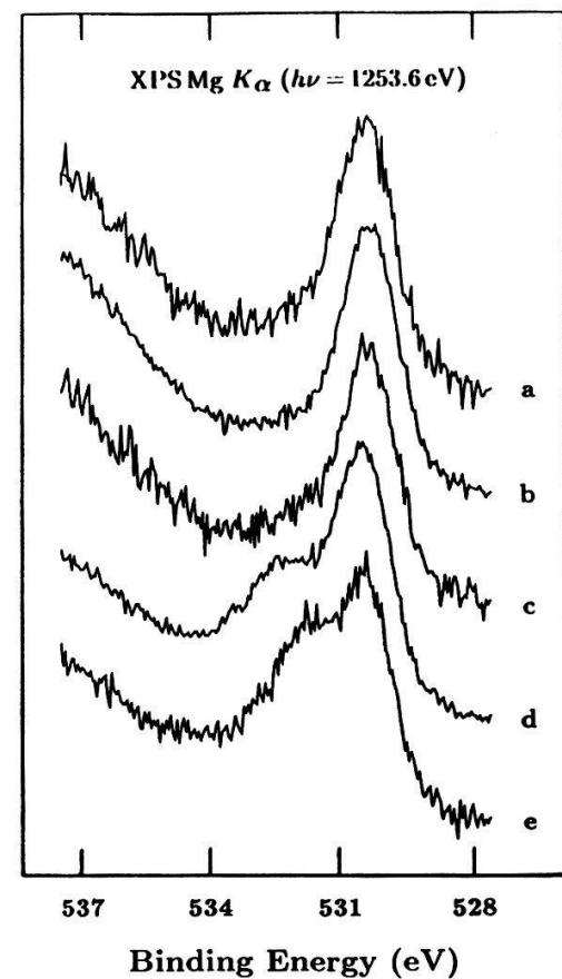
**Fig. 1b:** XPS O 1s core level spectra of a) 8 L  $\text{O}_2/\text{Ni}_{64}\text{Zr}_{36}$  at 300 K b) 8 L  $\text{O}_2/\text{Ni}_{64}\text{Zr}_{36}\text{H}_{34}$  at 300 K c) 8 L  $\text{O}_2/\text{Ni}_{64}\text{Zr}_{36}\text{H}_{34}$  at 300 K annealed to 400 K d) 8 L CO/ $\text{Ni}_{64}\text{Zr}_{36}\text{H}_{34}$  at 77 K annealed to 400 K e) 1 L  $\text{H}_2\text{O}/\text{Ni}_{64}\text{Zr}_{36}$  at 200 K.
