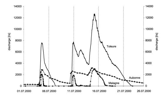
Fig. 4. Respective flood events for Aubonne, Toleure and Malagne springs in July 2000. The temporary spring of Toleure acts as a first overflow of the perennial Aubonne spring. Malagne spring starts flowing only during major discharge events. The discharge is determined after water levels measured at intervals of 4 hours at Aubonne, 30 minutes at Toleure and between 1 and 4 hours at Malagne.
