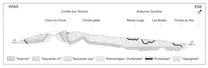
Fig. 2. Representative geological cross section within the Aubonne catchment area (adapted after Falconnier 1931). A perched aquifer is outlined within the Amburnex syncline (light grey).
