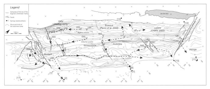
Fig. 7. Structural map of the top of the Oxfordian marls (adapted after Aubert et al. 1979, Falconnier 1951 and Lagotala 1920) and proposed limits of the catchment area of the Aubonne spring. This catchment area, based on structural criteria, is in good agreement with measured water balance and tracing experiments. Results of the tracer tests allow a first schematization of the main flow routes.
