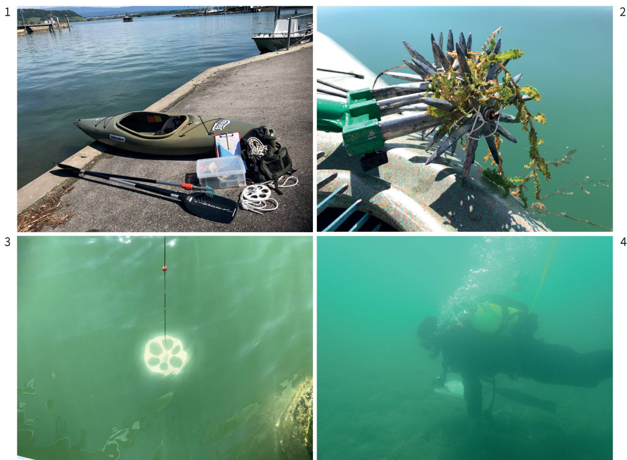
Figures 1-4. 1. Kayak with material for investigation. 2. Grapnel. 3. Secchi-disk. 4. Scuba-diver during investigation. Photos: A. Schwarzer.
