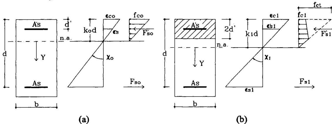
Fig. 1 - (a) Undamaged section ; (b) Damaged section
