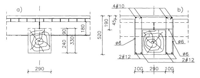
Fig. 2. Strengthening construction
