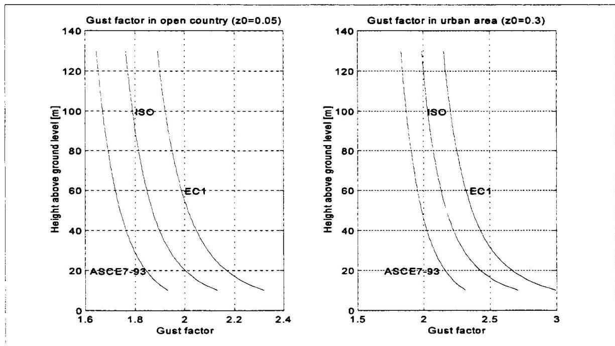
Fig. 2. Gust factor for velocity pressure averaged on 10 min,  $C_{gust}(z)$ .
