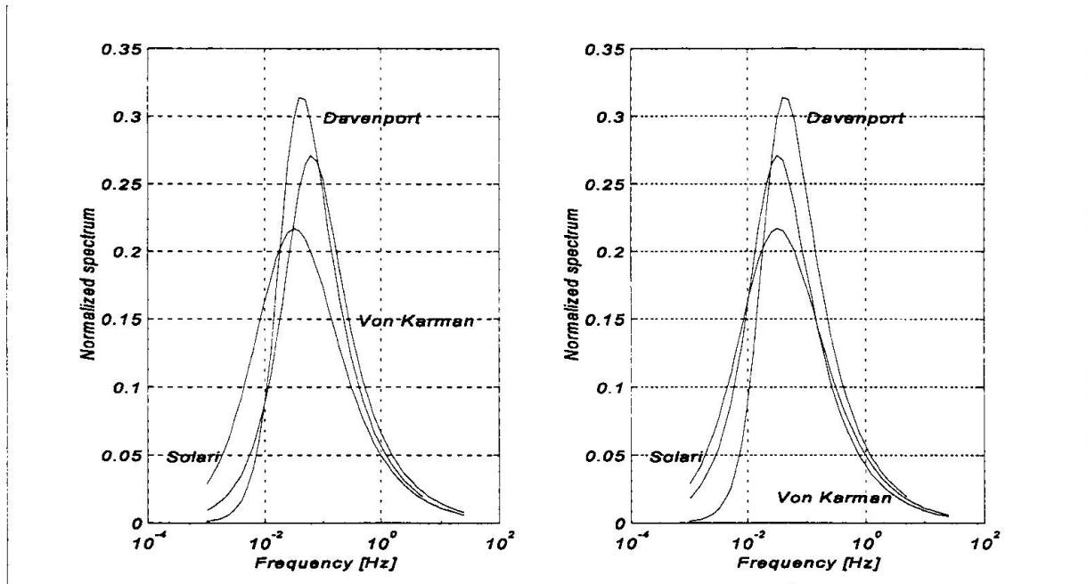
Fig. 4. Davenport, Solari and von Karman spectra at  $z=10m$ ,  $z_0=0.05m$ ,  $V_{ref}=30m/s$ , with 2 lengths of integral scale of turbulence in the von Karman spectrum; left:ESDU, right:Counihan.
