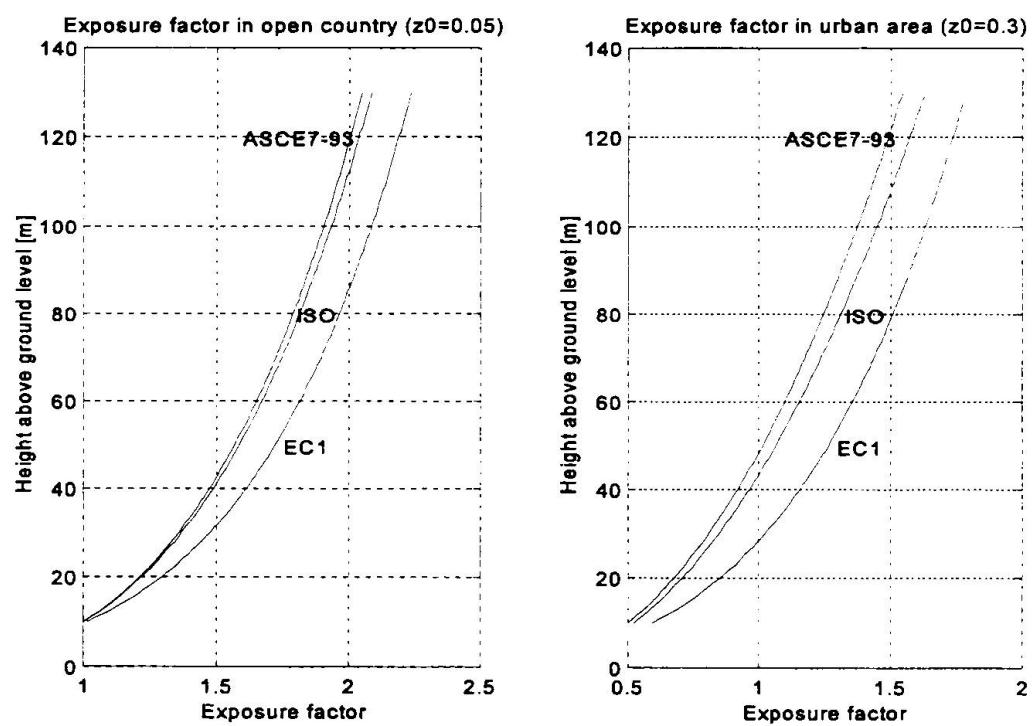
Fig. 1. Exposure factor (ASCE, ISO) or roughness factor (EC1),  $C_{exp}(z)$ .
