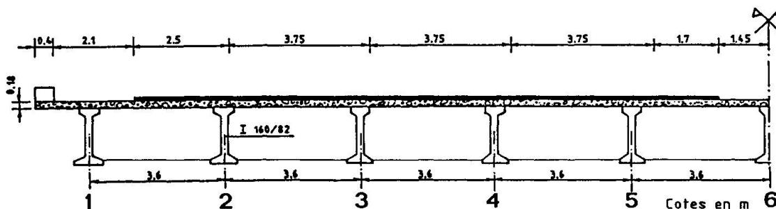
Figure 3 : Cross section of a Belgian bridge.
