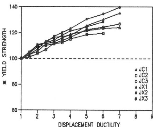
Fig. 6 Cyclic load-carrying capacity of the specimens
