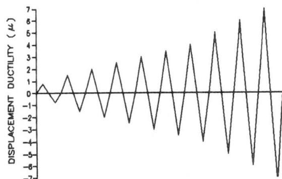
Fig 3 Cyclic load sequence used in the tests
