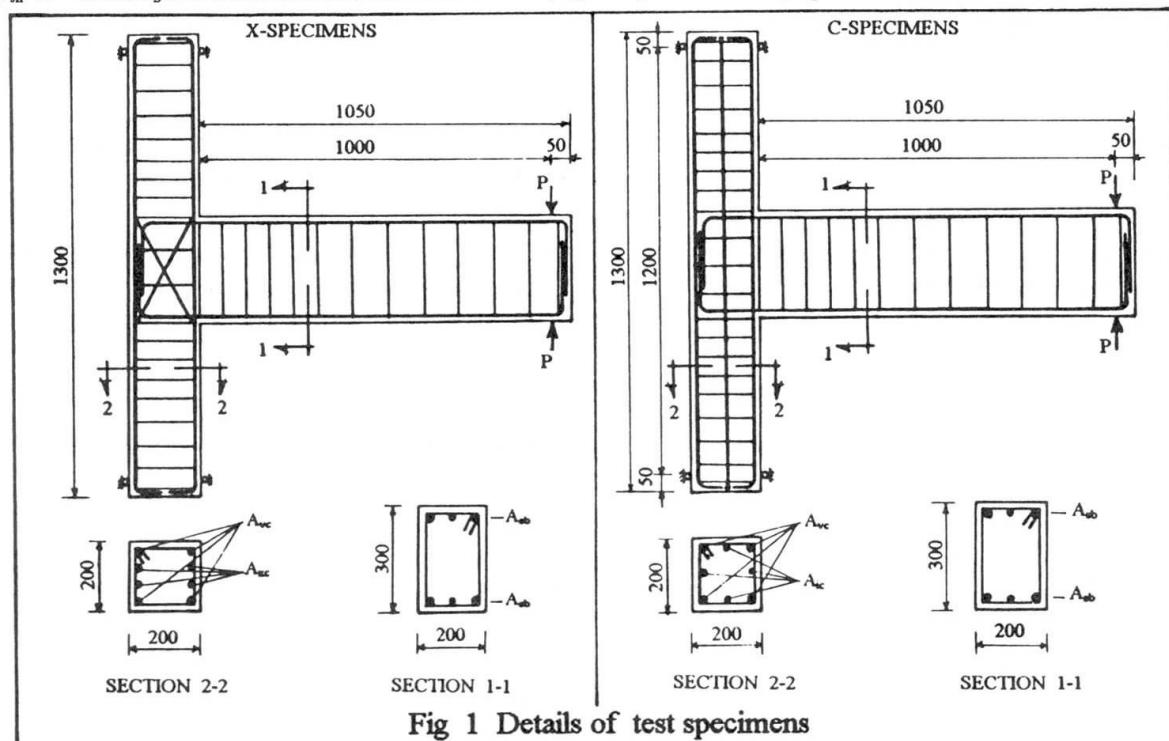
Fig 1 Details of test specimens
