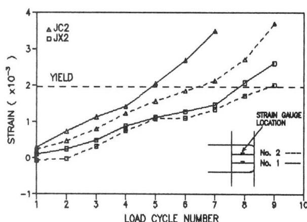
Fig. 7 Maximum strain in joint core hoops of specimens JC2 and JX2 during the positive loading runs of each cycle
