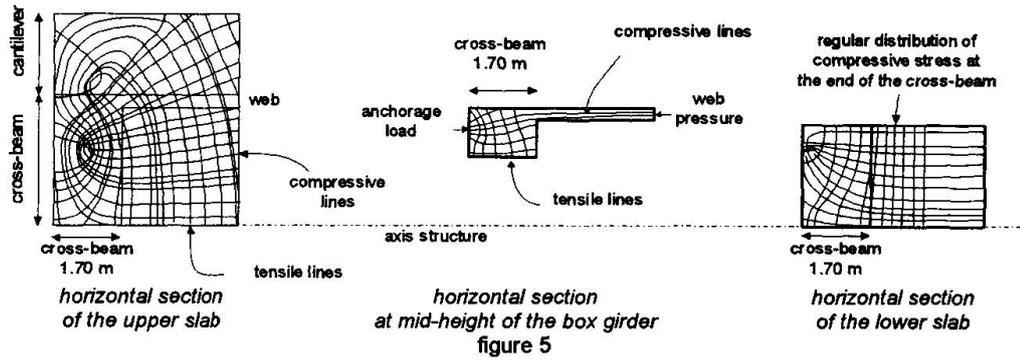
When the deformation of the part is visualized, the zones under greatest tension, exactly where the cracks occurred, are revealed. These areas are the back of the upright and the outside of the web (figure 6). We observe a "banana" shaped curvature of the uprights which explains why the web cracks occurred on the outside of the box girder and not the inside. Moreover, on these outer sides, more thermal and shrinkage effects are superimposed, resulting in more extensive cracking.
