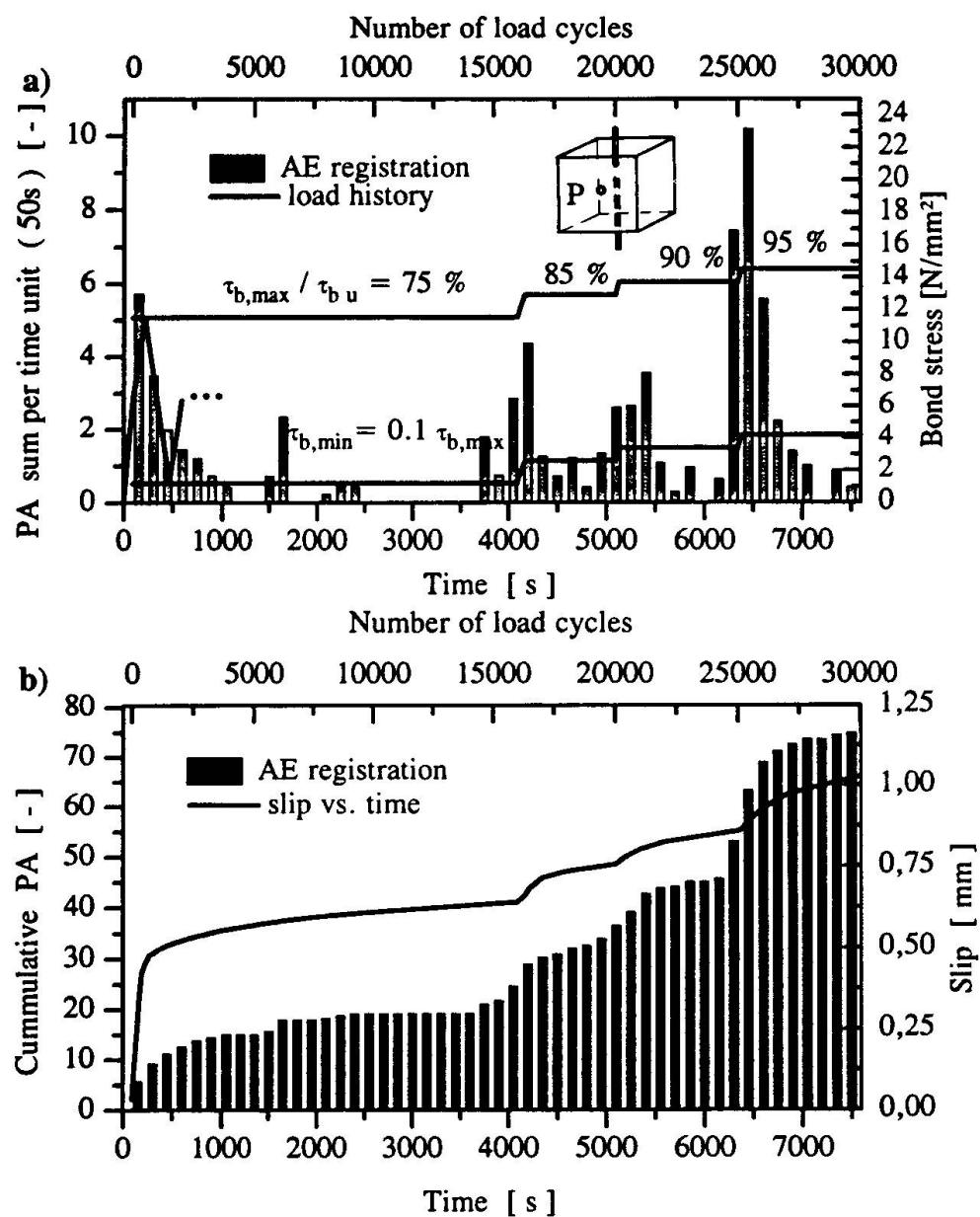
**Fig.4** Cyclic pull-out test with four load levels
