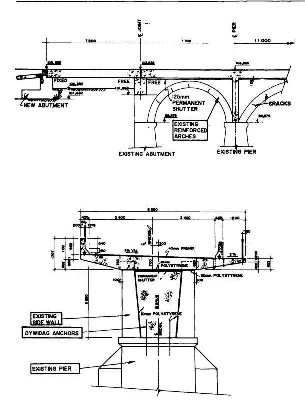
FIGURE I TYPICAL SECTION The new piers were designed as pinned joints resting on the existing piers and fixed by means of unstressed Dywidag bars grouted into the existing concrete. To ensure a minimum load transfer onto the existing structure, care was taken in providing for movement gaps between the old and new structure.
