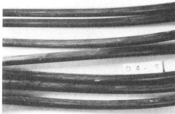
Taking into account the available test devices, twelve products were being tested by the LCPC at Nantes during 270 days, the left three products by the LCPC at Paris during 6 months for the first series and 31 months for the second test series with and interruption of one month after 22 months. For all the protection products, we observed that they bring an increase in the life time of the strands in the standardized stress-corrosion test conditions (NF A 05-302).
