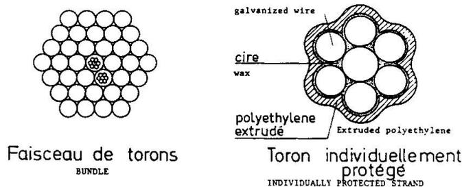
One may notice that steel protection is achieved quite early in the strand fabrication process, therefore preventing any chance of corrosion between successive operations. As soon as it leaves the factory, the "individually protected strand" product is therefore perfectly waterproof and efficiently protected against environmental attack.
