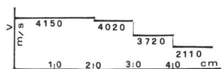
Fig. 3. Decrease of ultrasonic pulse velocity for increasing path length (detecting intermediate cracks)
