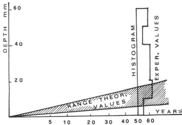
Fig.5. Carbonation depth vs time;
