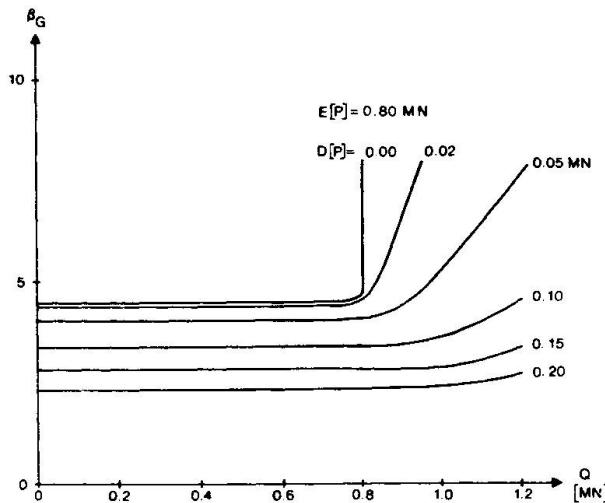
Figure 5: Reliability index  $\beta$  against the test load  $Q$
