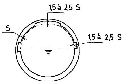
**Fig. 1** Schematization of the deterioration of the pipe-wall
