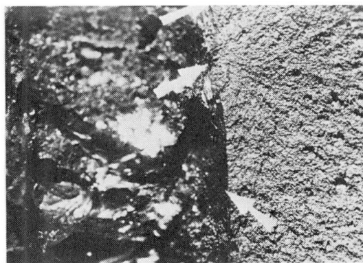
Photo 2 Fatigue crack at the notch of bridge No. 248
