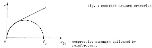
Here  $\tau$  is the shear strength and  $r_{fy}$  is the compressive stress, r being the reinforcement ratio.
