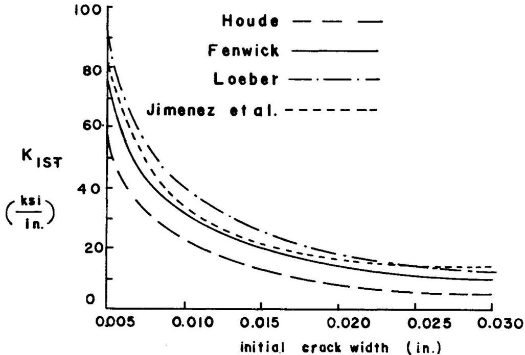
Fig. 13. Crack Shear Stiffness - Crack Width Relation (17)
