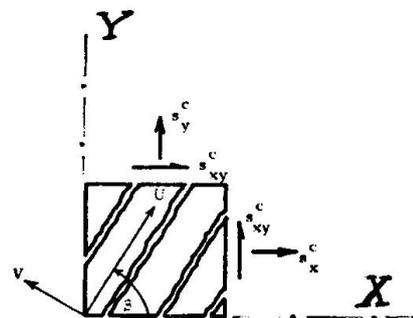
Fig. 4 Concrete Stresses in the Cracked Concrete
