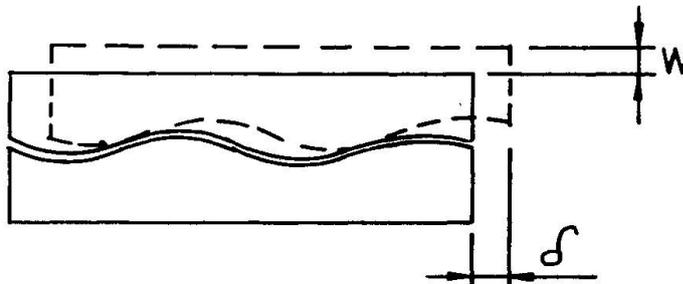
Fig. 11 Crack Displacements
