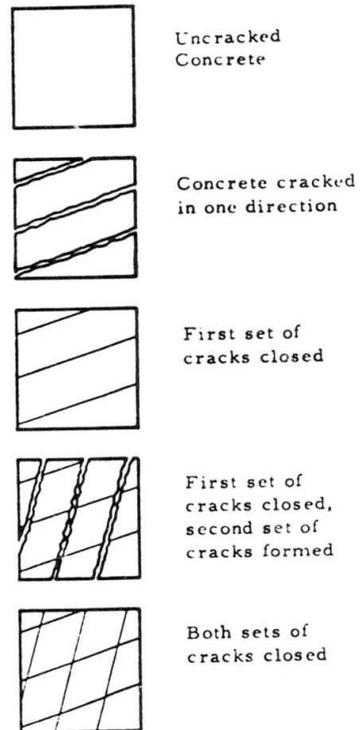
Fig. 5 Crack Modes
