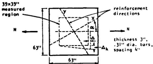
Fig. 8 Peter's Test Panel Subjected to Uniaxial Tension
