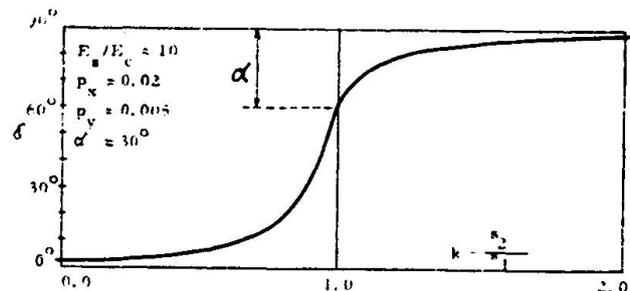
Fig. 7b Effect of Stress State on the Deviation of Concrete Principal Directions
