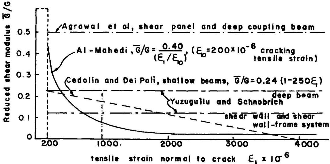
Fig. 15. Shear Stiffness Reduction in Cracked Concrete (20)
