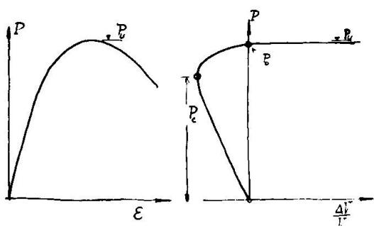
Fig.1 Stress-strain diagram and volume-strain-stress diagram
