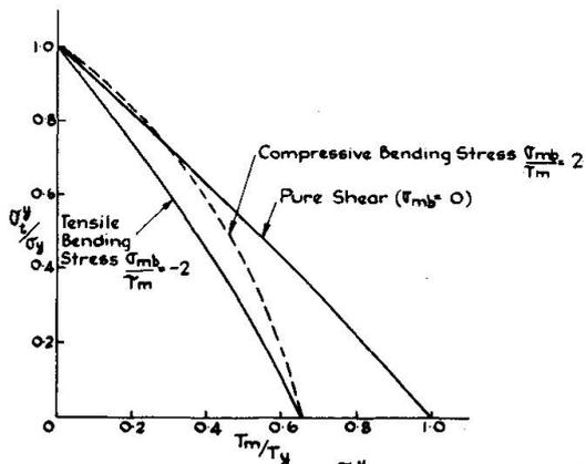
FIG. 8 VARIATION OF  $\frac{\sigma_t^y}{\sigma_y}$  RATIO WITH  $\frac{T_m}{T_y}$  RATIO
