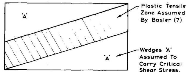
FIG. 3. COLLAPSE MODE ASSUMED IN BASLER THEORY.
