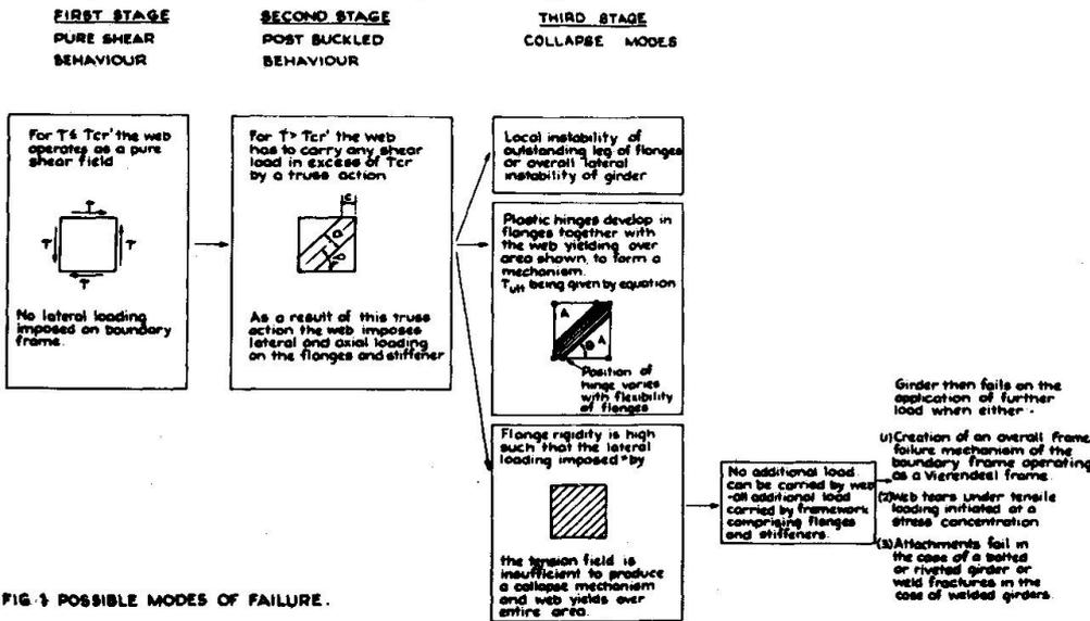
FIG 1 POSSIBLE MODES OF FAILURE.
