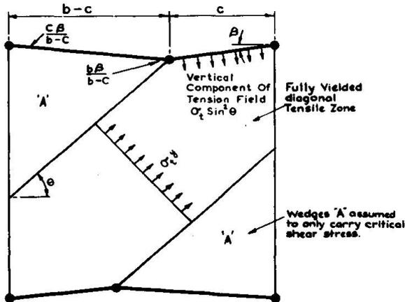
FIG. 2. COLLAPSE MECHANISM PROPOSED BY ROCKEY & SKALOUD (3)
