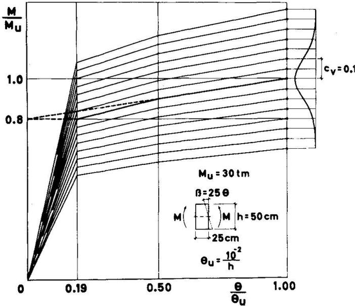
Fig. 2 — Trilinear moment-curvature diagrams.
