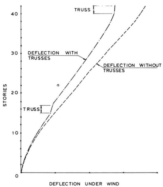
Fig. 4b Effectiveness of trusses in lateral resistance
