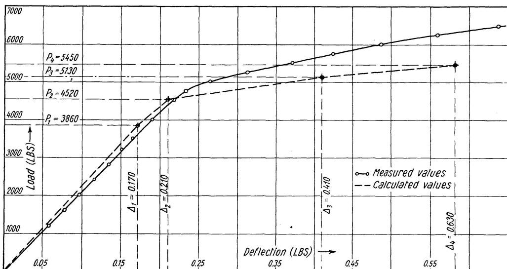
Fig. 6. Load-Deflection Curves at Mid-span of Longitudinal (2).
